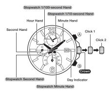
In the above sample illustration, the stopwatch shows an elapsed time of 20 minutes and 41.19 seconds.
